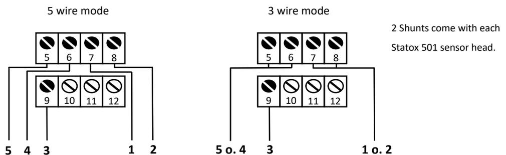
Figure 26: Connections sensor heads Stattox 501 HRC, ARE, LCIR, MCIR, CO<sub>2</sub> and PID
