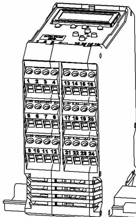
Figure 7: Pluggable terminal blocks with terminal numbers
