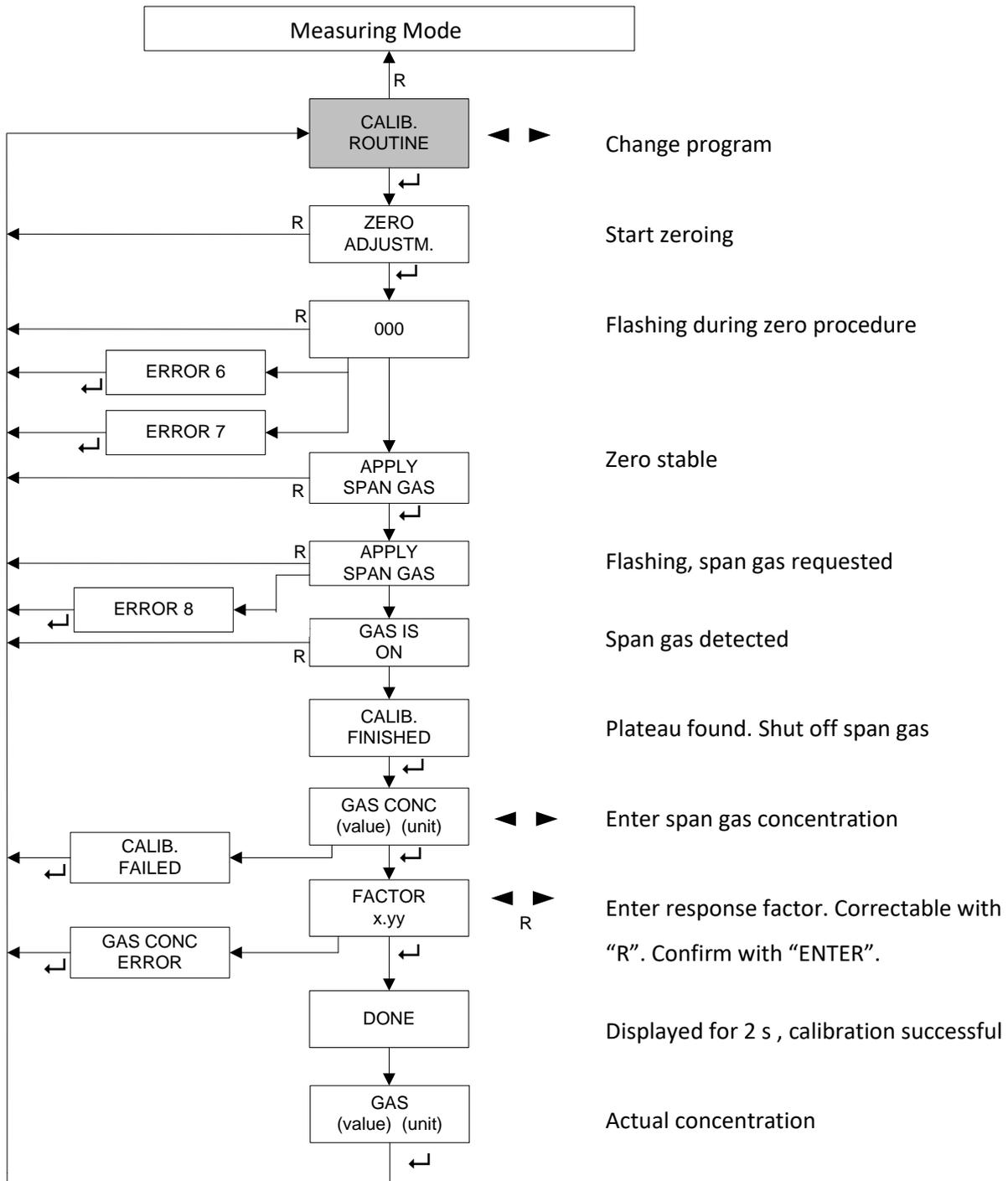
Figure 15: Calibration menu diagram
