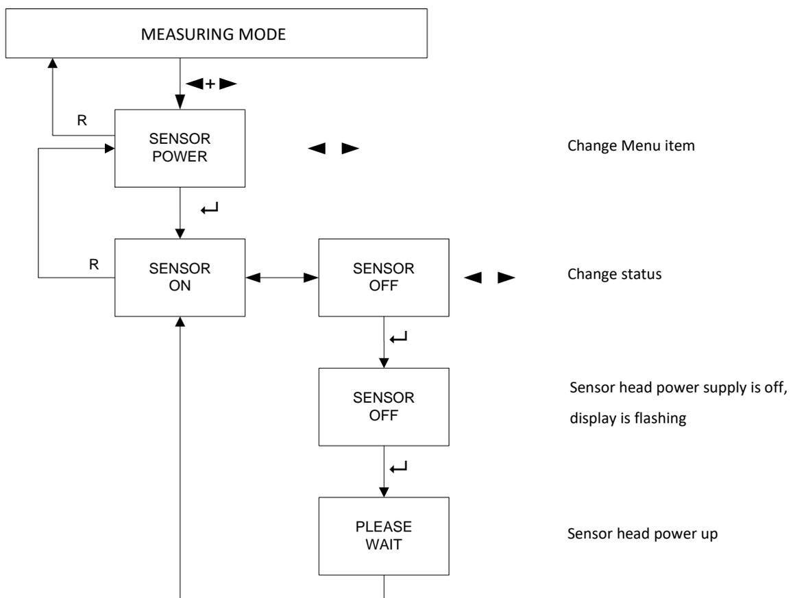
Figure 17: Diagram sensor head deactivation
