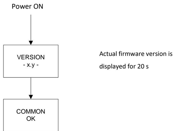
**Figure 19: Start procedure in Common Alarm mode**
