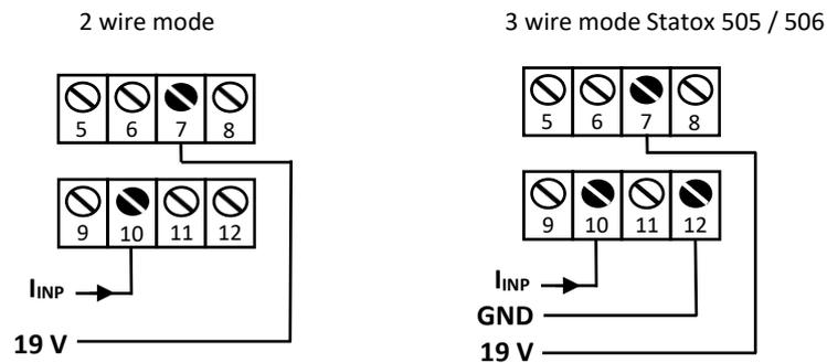
Figure 24: Connections sensor heads Stattox 501/S, Stattox 505 and Stattox 506
