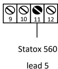
Figure 9: Stattox 560 Self Test Trigger Connections
