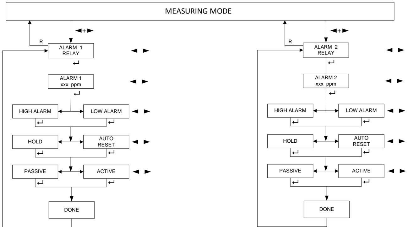
**Figure 18: Control Module - alarm relays setting**
