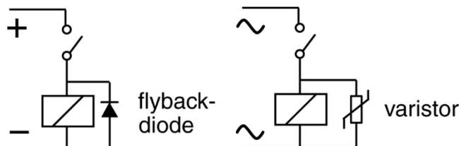
Figure 11: Left: Flyback diode in a DC circuit to prevent voltage peaks, Right: Varistor in an AC circuit to protect against overvoltage.
