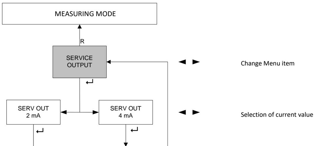
**Figure 22: Diagram service output**
