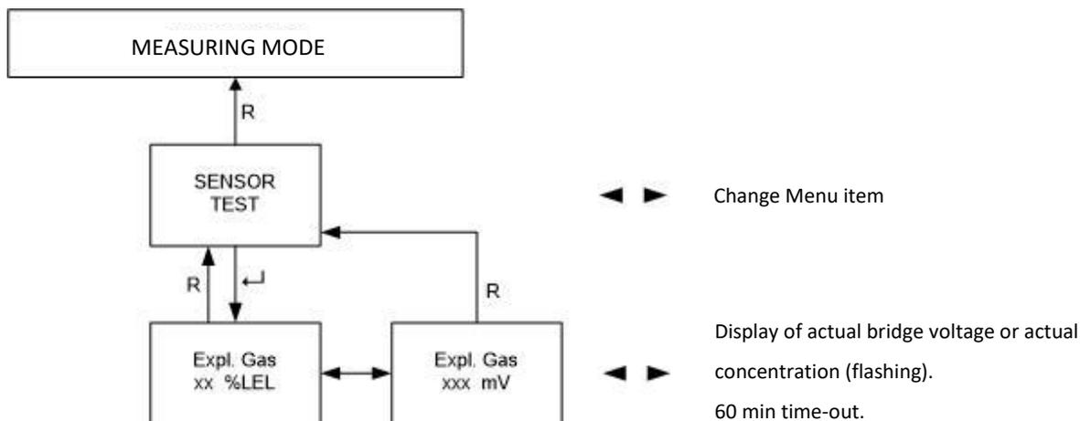
Figure 16: Sensor test menu diagram
