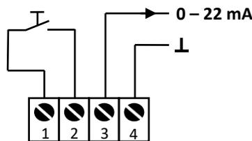
Figure 8: Connections external reset and analog output
