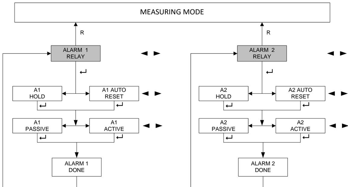
**Figure 20: Common Alarm Module - alarm relays setting**
