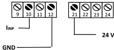
Figure 25: Connections sensor head Stattox 501 Infratox / Infratox HS
